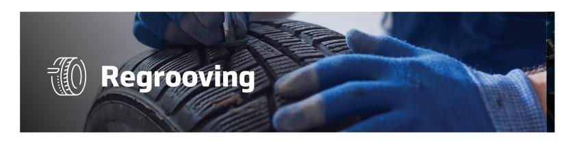
A regrooved tyre is a tyre, either new or retreaded, on which a tread pattern has been produced by cutting into the tread in accordance with the tyre manufacturer's regroove tread pattern. By regrooving your premium Hankook tyres you save resources, preserve the environment and save yourself money on tyres and fuel.
