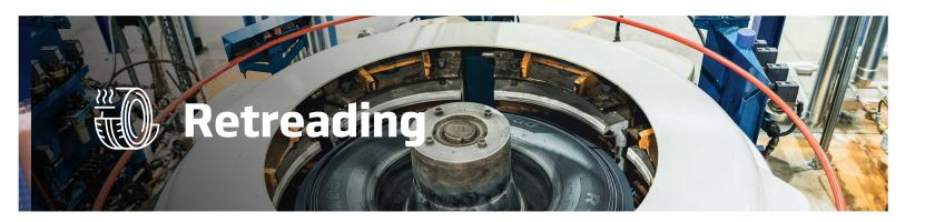
Hot cure retread is a re-manufacturing process for tyres that replaces the old tread with a new tread to extend the life of the tyre. Hankook Alphatread hot-cure retread tyres can deliver up to 100% new tyre mileage and on-road performance at around 70% of the cost of a new tyre.
